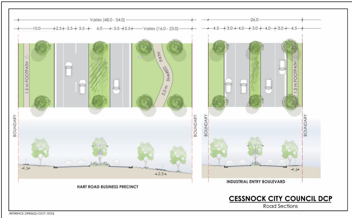
Figure 12 - Road sections: Business and industrial entry boulevard
