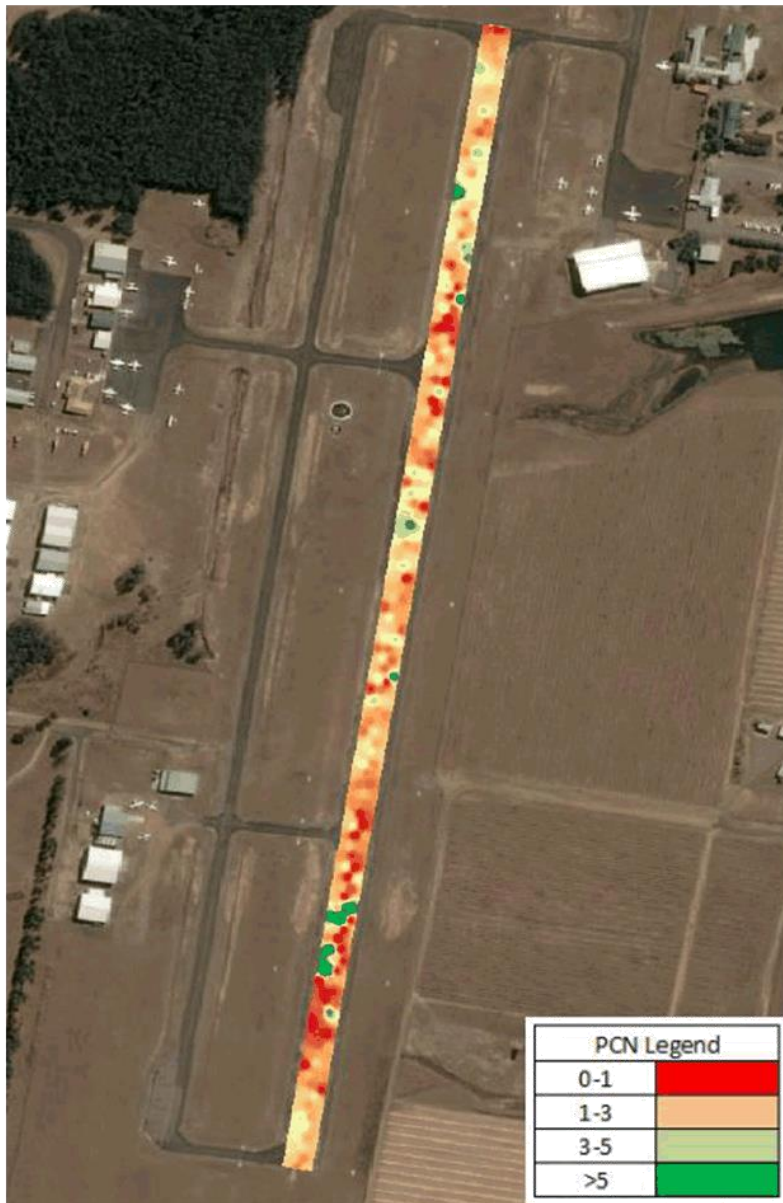
Figure 2-7 Runway Pavement Strength (PCN) Heat Map Source: Pavement Management Services, 2018
